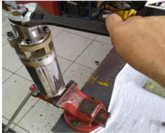
Figure 14 –Drive Fixed Pump for Unscrewing Plastic Part
