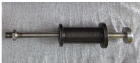
Figure 7 - Interchangeable withdrawal shaft
