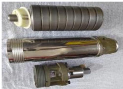
Figure 15 - Disassembled Pump
