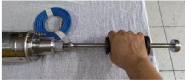
Figure 11 - Tool Kit Coupled to Pump Motor Cover
