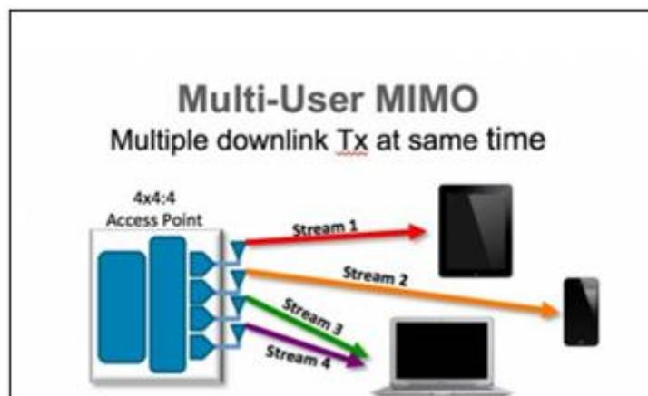
Figure 2 - Scheme of using MIMO technology
