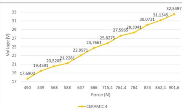
Figure 2 - Voltage Generated as a function of Applied Force
